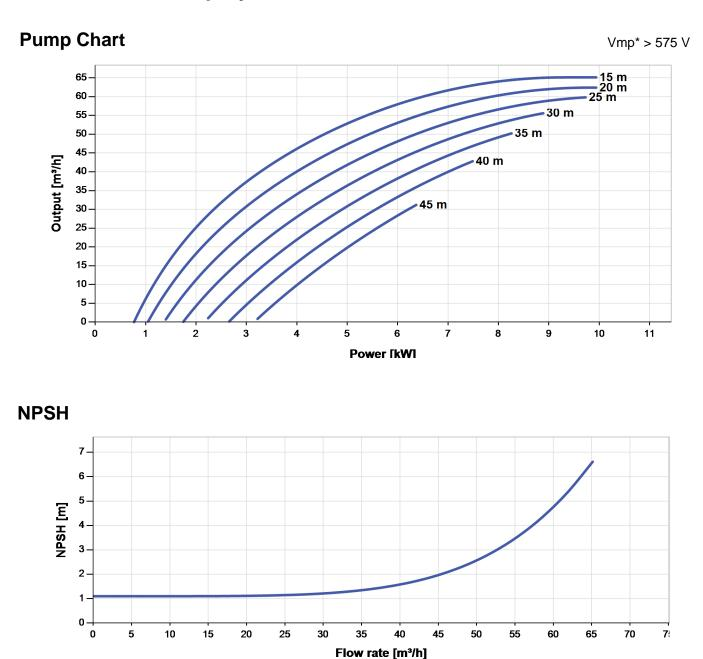
The NPSH (Net Positive Suction Head) is NOT the operating suction head. To calculate the operating suction head please refer to the installation manual.
